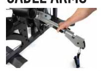
To adjust the functional cable arms simply squeeze the handle with one hand. With your other hand adjust the cable arm up or down until the cable arm is in the desired starting position. Then release the handle to secure the cable arm in place.
