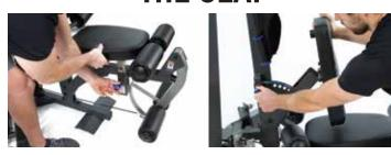
Adjust the seat height by loosening the pop pin, then pull the pop pin out with one hand and raise or lower the seat with your other hand. Release the pop pin and tighten.
