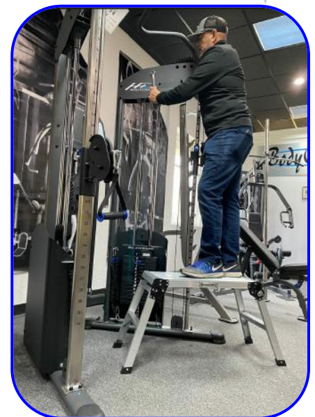
Example picture of using a Step Platform to work on assembly above 5' tall areas.
