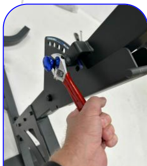
Fully tighten Pop-Pin with Adjustable Wrench.
