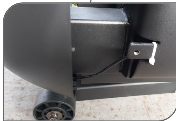
Picture above for routing reference, DO NOT secure cable at this time.
